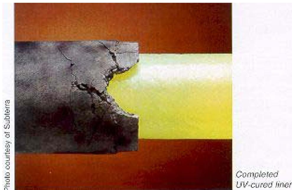
Typical curing times are between 0.5 and 0.9 m/min, and lengths of up to 200 m can be lined continuously. UV-cured systems are available for pipes from 100 to 1,000 mm diameter, with liner wall thicknesses from 3 to 15 mm. Variations are under development to line lateral connections.
