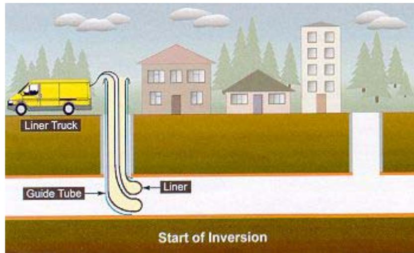
Insertion into the existing sewer is usually carried out either by winching into place or by an inversion process wherein water (or sometimes air) pressure is used to turn the liner inside out as it travels along the pipe. The following procedure is typical:-
