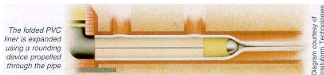
Once inserted, the pipe is heated using a hot air tool, which activates the shape memory of the material and causes it to revert to the size at which it was extruded. The liner pipe expands to achieve a close fit, moulding itself to any intrusions and joints. If, prior to reversion, the host pipe is broken out at the position of branch connections, the new pipe expands to the correct dimensions for the use of standard electrofusion fittings.
