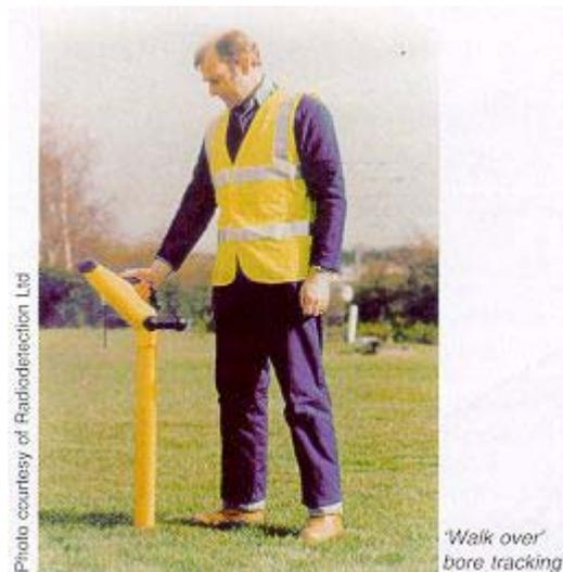
*A walkover system tracking an HDD bore. Picture courtesy of Ditch Witch/ Subsite.*
