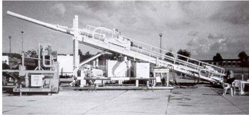
*Large directional drilling rig designed for long-distance crossings beneath major rivers, estuaries, motorways, railways and canals*
