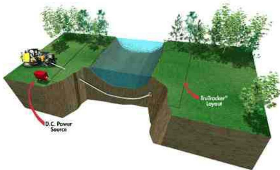
*Artificial magnetic field set up in high interference areas for HDD hard wire guided bores. Picture courtesy of Inrock Drilling Systems*
