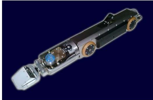
A typical Grinding Robot with onboard CCTV monitoring system.
