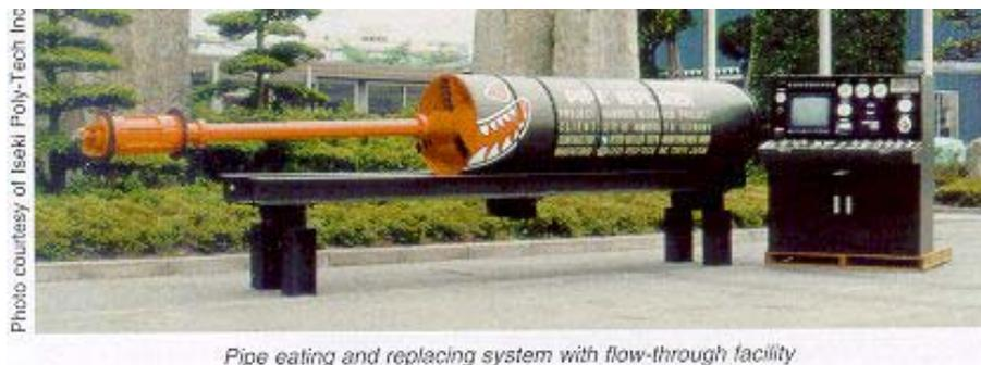
A further adaptation uses specially designed teeth within the cone crusher to cut the reinforcement in a concrete pipe, allowing the excavation of all conventional pipe materials in addition to concrete. Some machines have a pilot head fitted to the cutting wheel, which guides the machine within the existing sewer, together with pneumatic hammer action, which assists the cutting head to crush the old pipeline.
