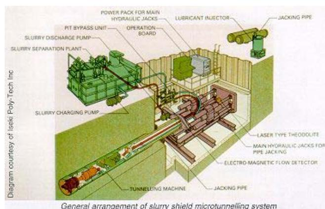
The slurry system has the advantage of being continuous, whereas auger-based methods which require the hoisting of spoil are more cyclical and involve interruptions to the operation of the cutting head.
