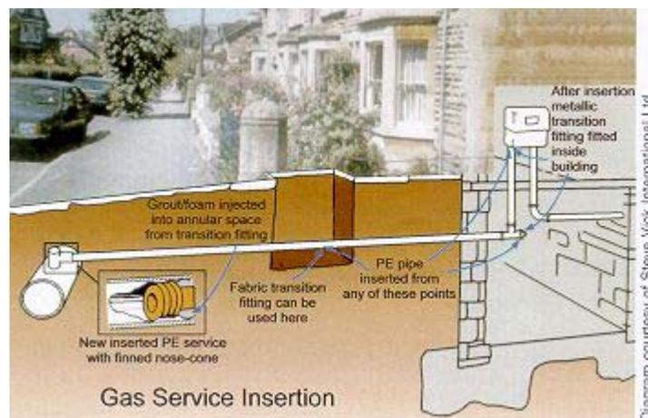
A method of live insertion for gas service pipes has been developed in which a new PE pipe is pushed into an old steel service through a gland sealing system attached to the old pipe, either inside the consumer's premises or by means of a small excavation
