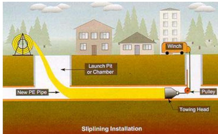
Small liners may be pulled in manually, but most need a winch. The winch should apply a steady, progressive pull, without snatching or uncontrolled variations in force. Careful consideration should be given to the positioning of the winch and the routing of the cable, and it is often necessary to fit additional pulleys within the manhole or reception pit, to ensure that the cable has an unobstructed path and does not abrade on any part of the chamber.
