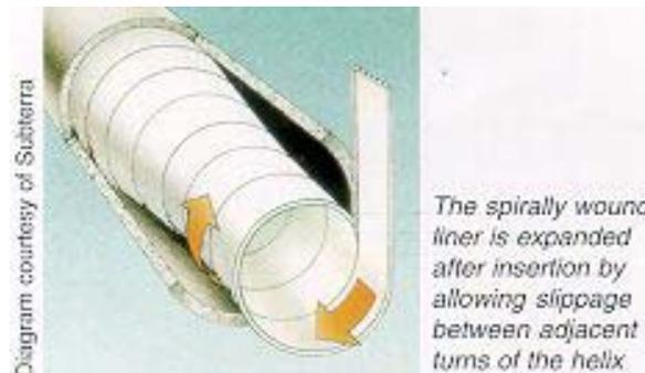
As with the standard form of spiral liners, low flows in the pipeline can be accommodated during installation without the use of overpumping or diversion. Since there is no grouting, groundwater may enter manholes by following the path between the outer T-beams. It is therefore essential to provide a good seal between the liner and the host pipe at chambers. Sealing must also be carried out at any lateral connections.
