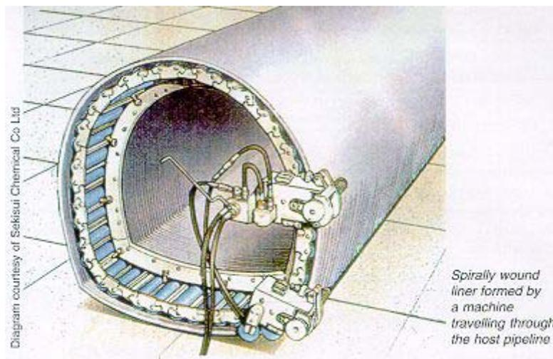
The profile has a ribbed outer surface in the form of 'T-beams' which increase the structural strength of the tube and also provide a mechanical bond with the grout injected between the liner and the existing pipe wall. The inner surface of the tube has a low roughness coefficient, and the material resists most chemicals. In some systems, steel reinforcement can be inserted between the profile ribs prior to winding, to increase the strength of the tube.
