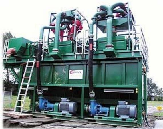
*A typical microtunnelling spoil separation and fluid recycling set-up.
