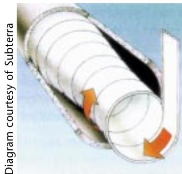
*The spirally wound liner is expanded after insertion by allowing slippage between adjacent turns of the helix*
