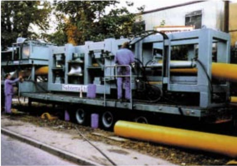
*Machine for simultaneously reducing the diameter of a PE pipe and inserting it into the host pipeline*
