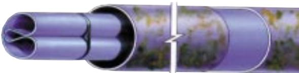
*The folded liner is inserted into the host pipe, and then reverted to its original shape*
