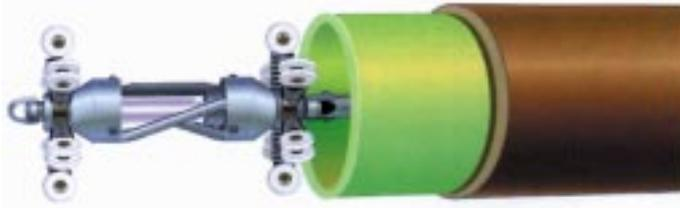
*The UV light source is pulled through the liner at a controlled rate, while internal pressure is maintained*
