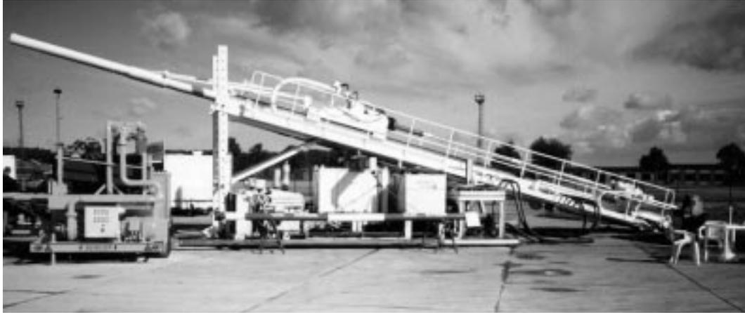
*Large directional drilling rig designed for long-distance crossings beneath major rivers, estuaries, motorways, railways and canals*
