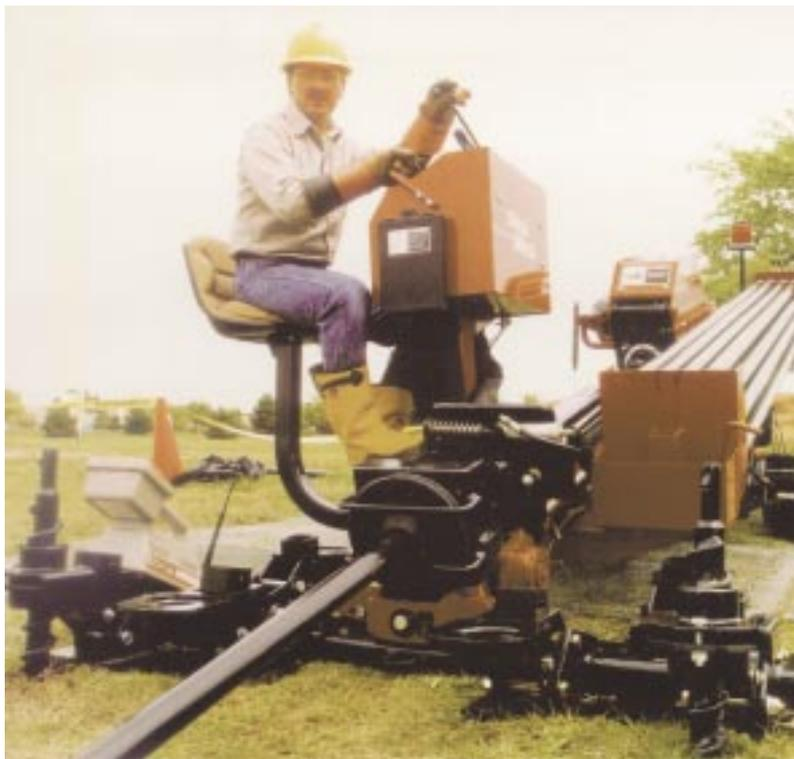
*Drilling the pilot bore with a typical surface-launched guided boring machine*
