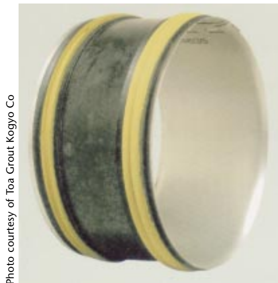
Stainless steel and rubber internal repair sleeve for gravity pipes, with additional hydrophilic rubber seals (yellow)
