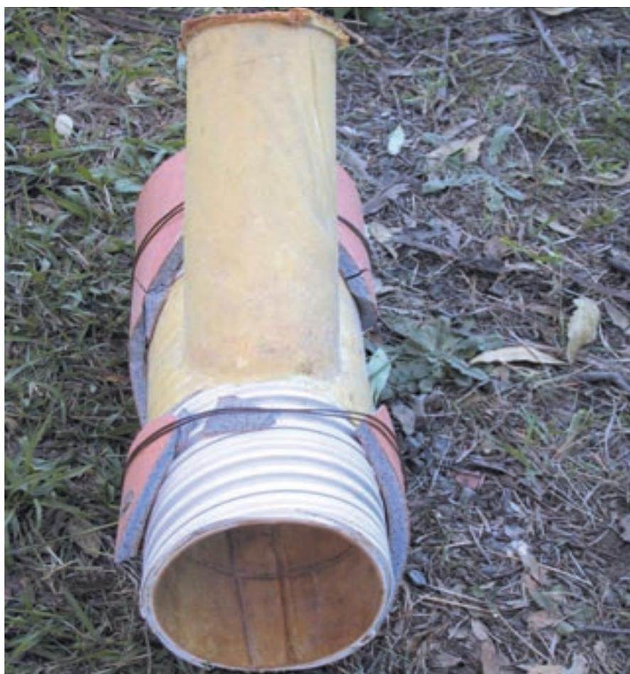
■ Interflow L.C.R. removed from a sewer junction following a trial installation. An effective physical barrier to root infestation has obviously been provided.
