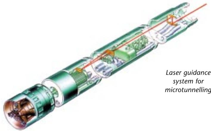
*Laser guidance system for microtunnelling*
