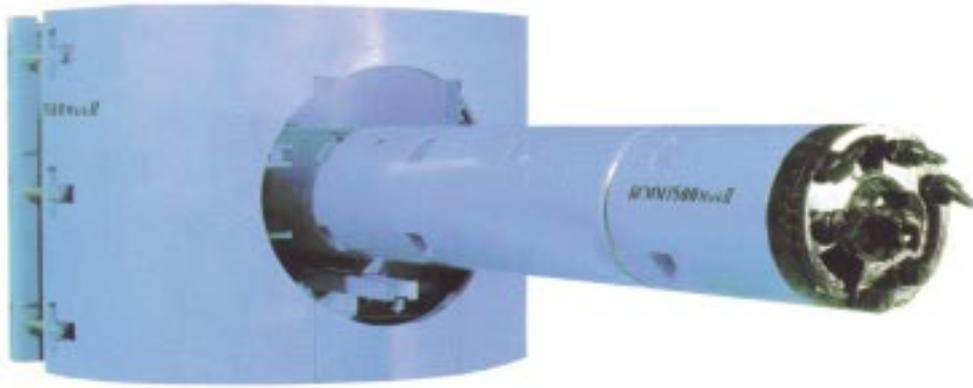
*Auger microtunnelling machine designed to operate from small-diameter shafts*
