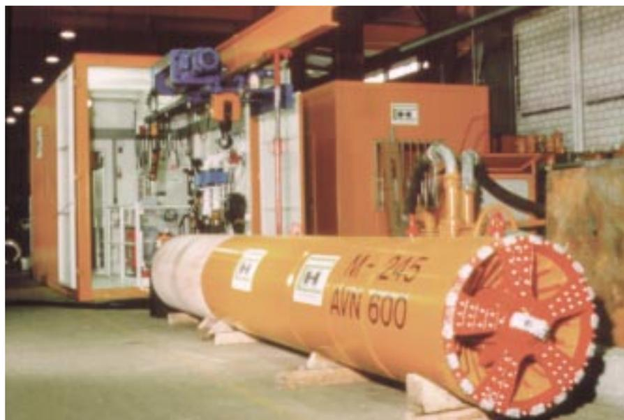
*Microtunnelling system with containerised power-plant ancillaries*
