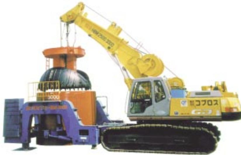
*Specialised system for shaft excavation, using a hydraulic 'clam-shell' bucket*
