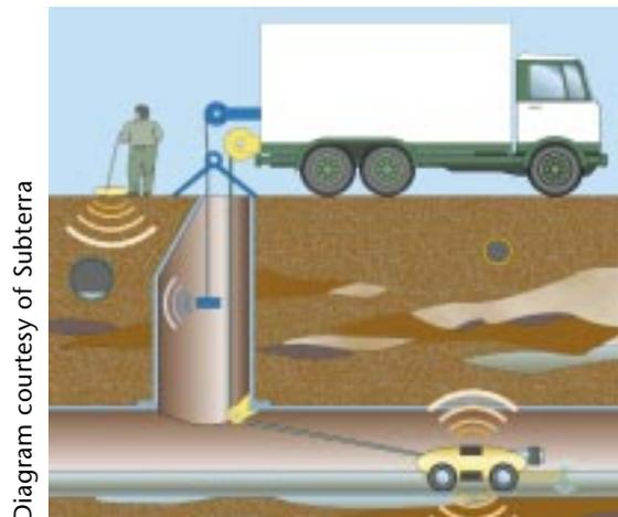
*Ground-penetrating radar may be used from the surface, or from within a chamber or pipe*
